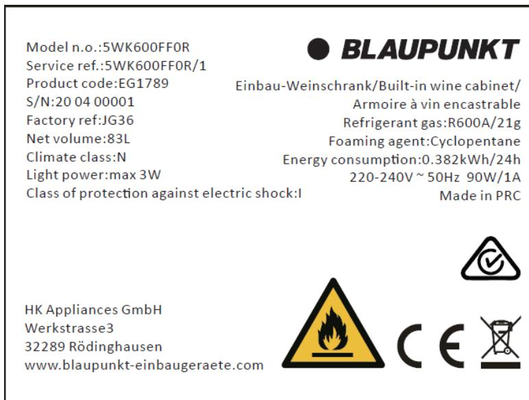
The nameplate attached to the inside or rear of the appliance (depending on the model) includes the entire information specific to your appliance.
