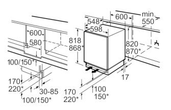
\* variable base/substructure height
