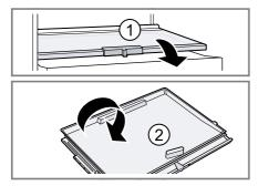
**3.** Press the fastenings for the lower cover outwards.
