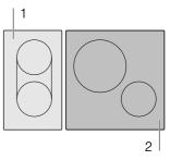
**Note:** In the combi zone, the PowerBoost function can only be activated if the two hotplates are used independently of each other.
