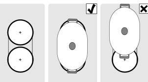
When you are using cookware on just one of the two hotplates, it can be moved to the second hotplate. In this case, the heat setting and the selected settings are transferred.
