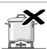
Do not use damaged pans, which do not sit evenly on the hob. Pans may tip over. Only use pans with a thick, flat base.
