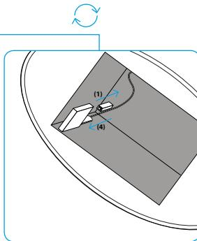
**Fig. 3 Simple receiver installation** The receiver can be installed easily without additional tools. Remove the cover frame from the **top** of the hood and insert receiver. Remove the stick (1) from the **inside of** the hood and insert the receiver (4).
