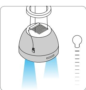
**Fig. 2 Installing the optional remote control of additional lighting features is simple.** Installing a receiver (Order Number: BLZ 501) and connecting it with the remote control (Order Number: BLZ 502) allows the colour temperature and brightness of the hood to be controlled.
