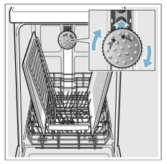
To ensure that the spray jet can reach all parts, arrange the baking sheets as illustrated (max. 2 baking sheets and 2 grilles).
