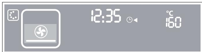
4. Touch the ☰ button and set the temperature using the rotary selector.
