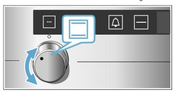
Use the temperature selector to set the temperature or grill setting.
